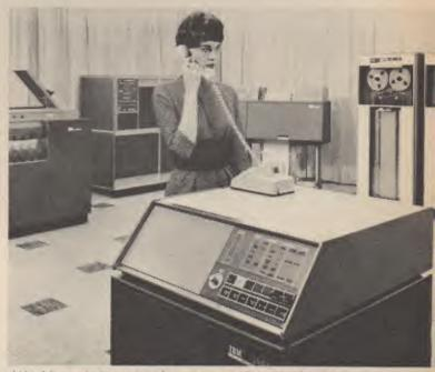
Would you believe it, when you saw it in a science fiction picture? The data transmission unit above enables computers to hold direct two-way telegraph or telephone "conversations." Or, to put it a little more specifically: the computer can send business or scientific information any distance directly from its magnetic memory to the storage of another computer. Here the operator dials the office across the country to make a connection for data transmission.
